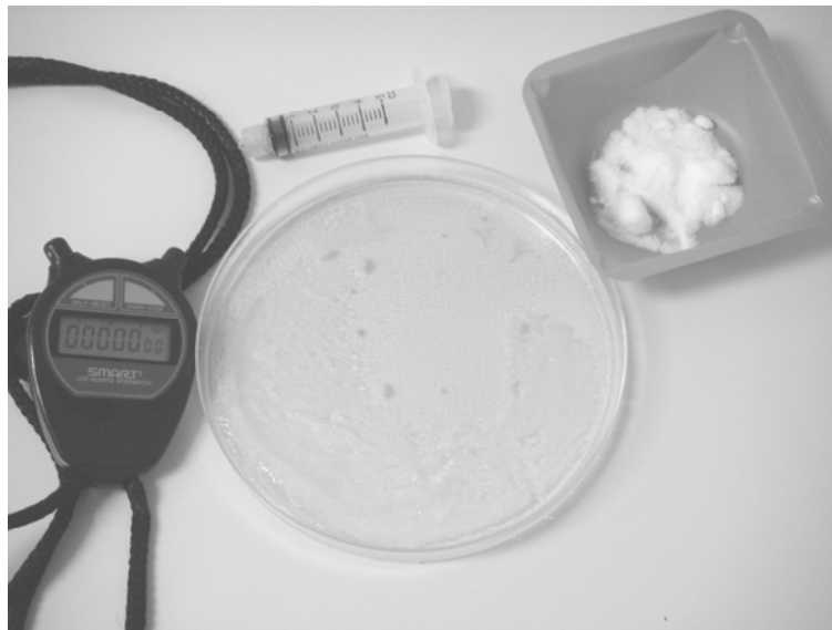
Figure 1 - Example of Ice Melting Test Set-Up
